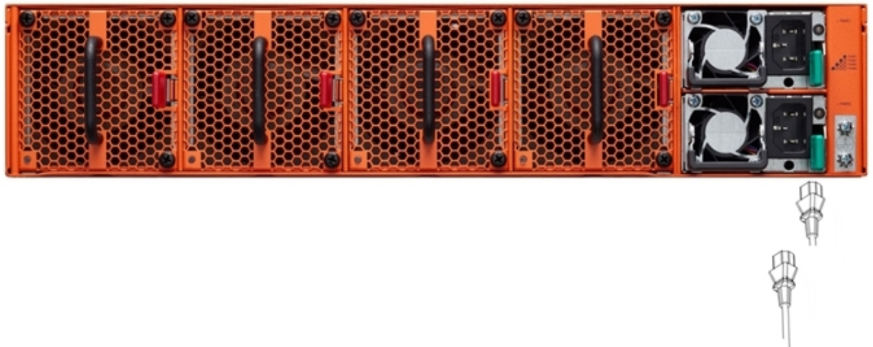
Figure 11 Connecting AC Power on a GigaVUE TA Series-TA200
